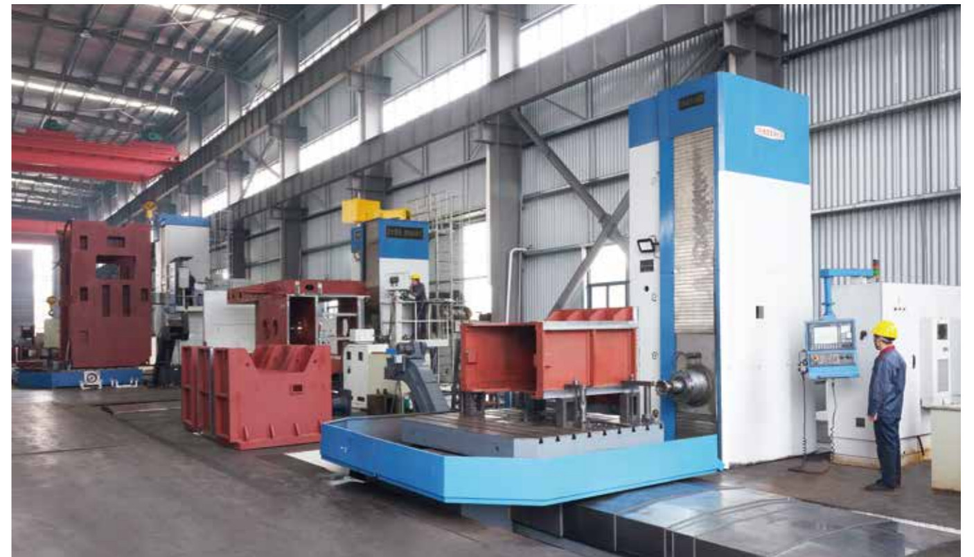
大型數控落地鏜銑床 Large CNC floor boring and milling machine
